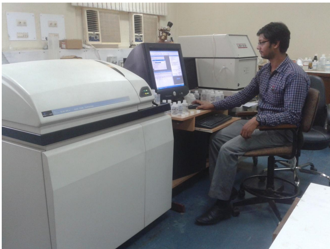
Figure 4.3: Author at work on ICPMS in Mass Spectrometer Lab at WIHG, for trace elemental analysis.
