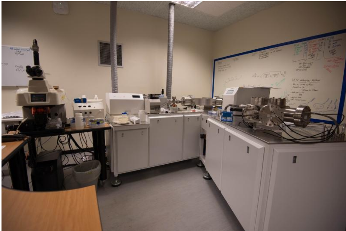
Figure 4.10: Photograph of MC-ICPMS facility (Nu Plasma) used in this study for Lead (Pb) isotope systematic at University of Cape Town, Cape Town, South Africa.
