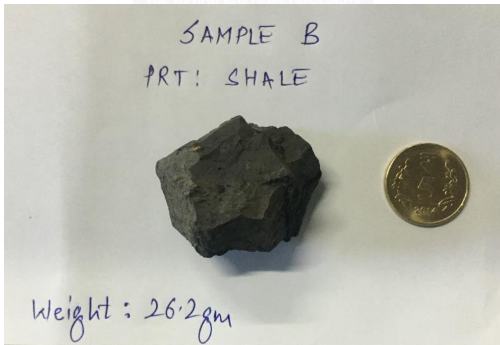
Fig16: Shale Sample B weighted before running demonstration
