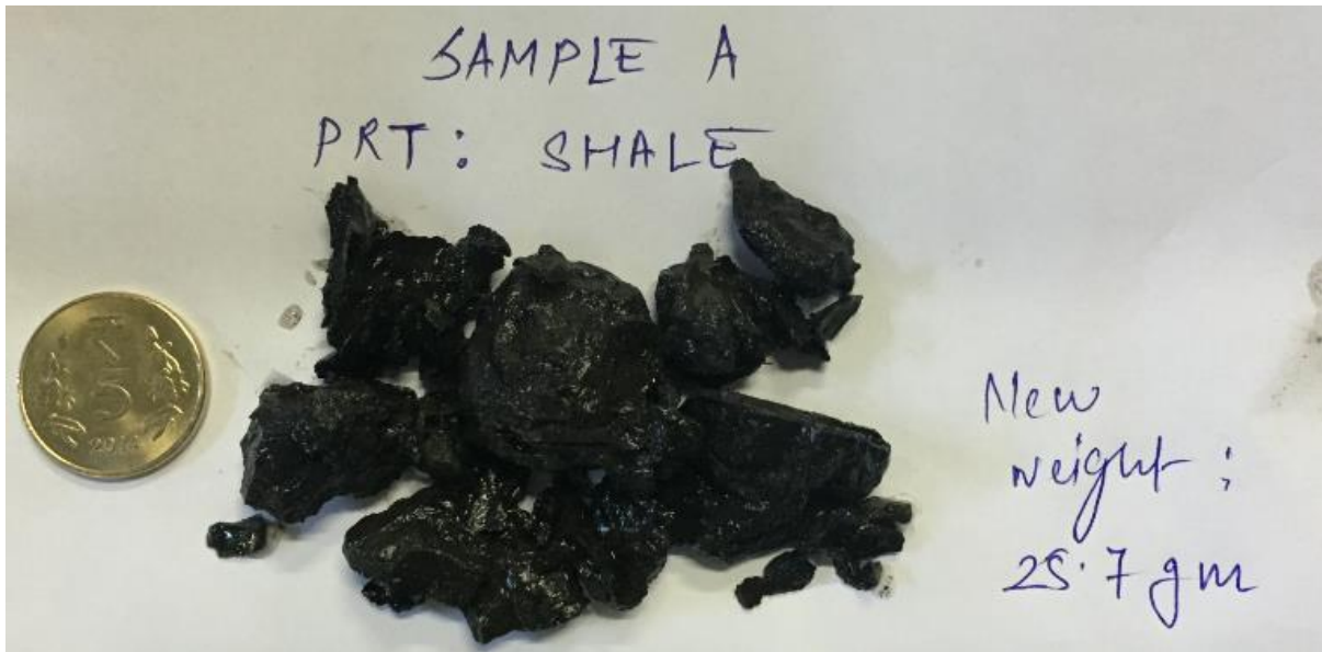
Fig19: Shale Sample A after running demonstration and new total weight
