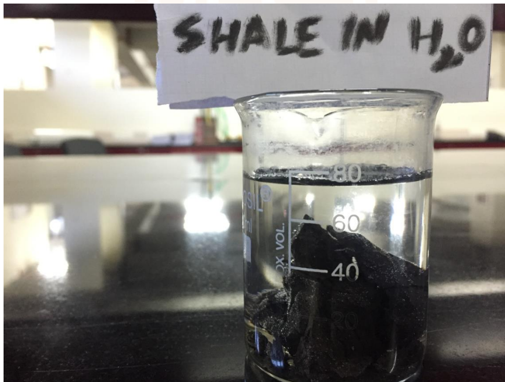
Fig18: Disintegration of Shale due to swelling clearly visible
