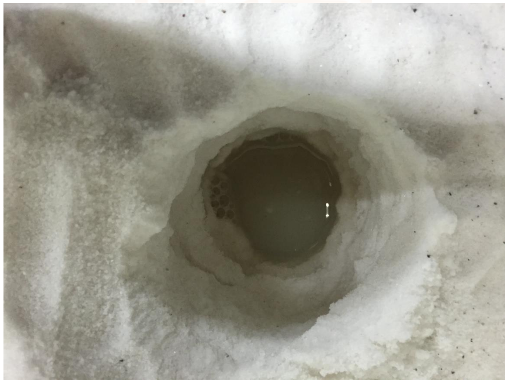
Fig22: Stable Gauge after injecting Salt Saturated Polymer Mud
