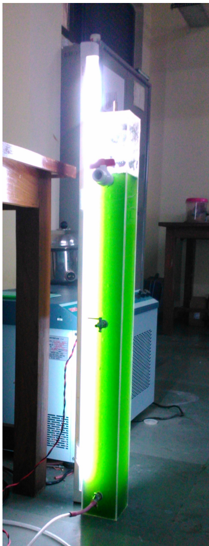
Figure 3.2: Photobioreactor of 10 lit capacity using Anaerobic digester as nutrient
