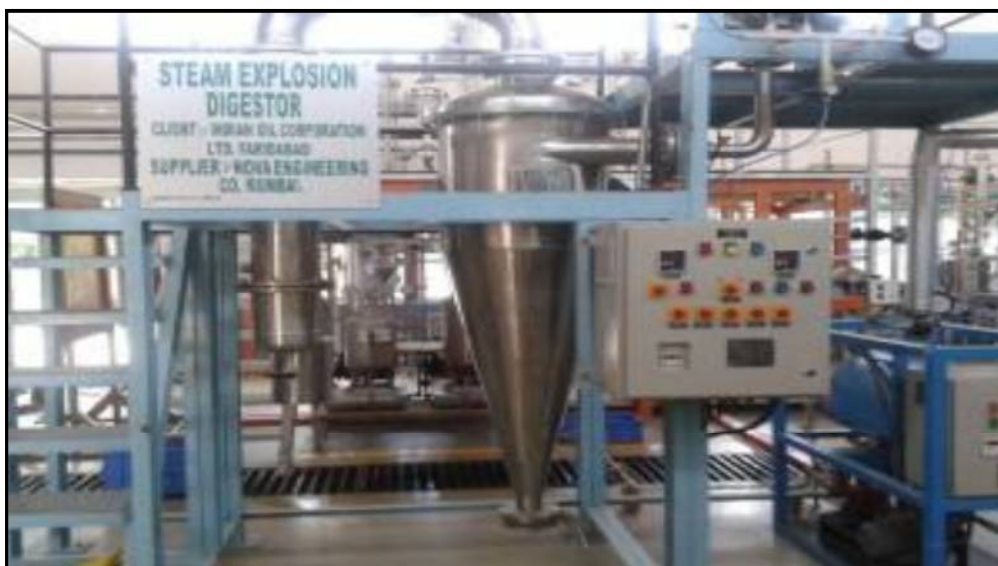
Figure 5.4 Lignocellulosic pilot plant based on steam explosion pretreatment
