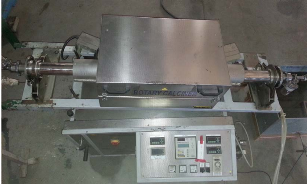
Fig. 3.5 Photograph of the rotary tubular helical coil gasifier experimental set-up
