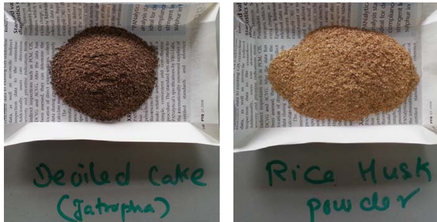
Fig. 3.8 Images of pulverized biomass samples of jatropha deoiled cake and rice husk
