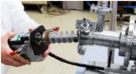
Fig. 3.6 Photograph of screw conveyor
