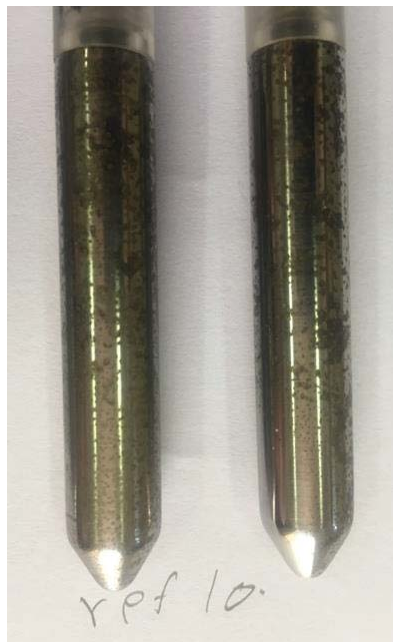
Figure 5.7: Worst rating of grade 'E' with very extensive corrosion pits on the spindle
