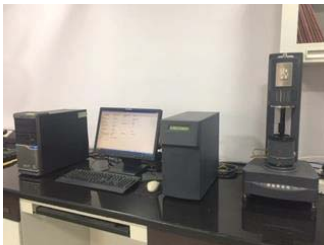
Figure 4.4: M/s TA make AR 2000Ex model Rheometer
