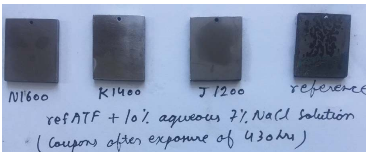
Figure 5.39: Coupons after testing with 10% volume of 7.0% NaCl after 430hours
