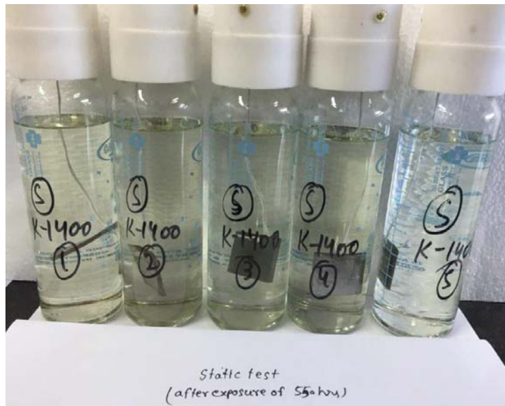
Figure 5.28: Test bottles containing coupons at the end of 550hours of static tests for 1400ppm of Karenjia
