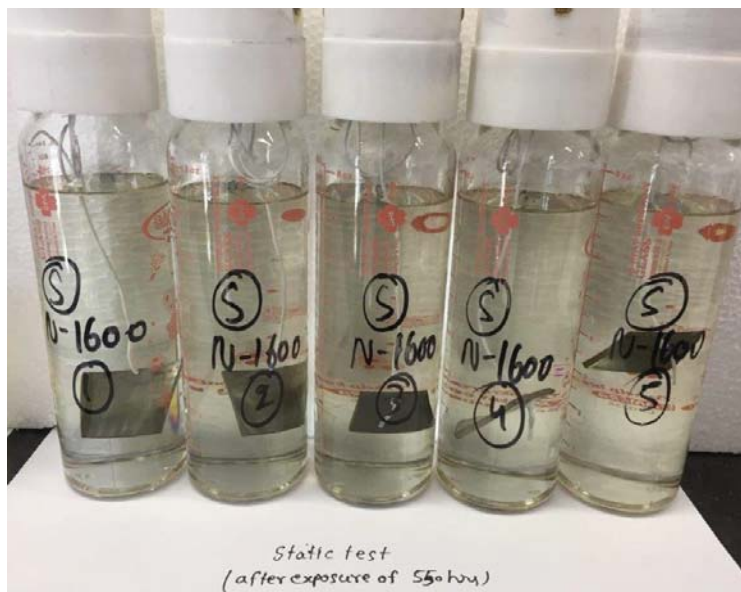
Figure 5.27: Test bottles containing coupons at the end of 550hours of static tests for 1600ppm of Neem
