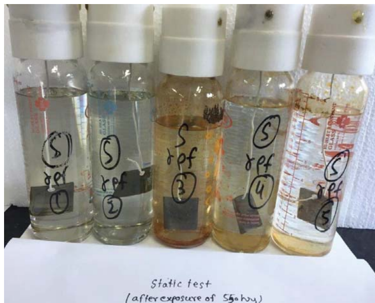
Figure 5.29: Static test bottles of reference ATF with coupons at the end of 550hours of exposure
