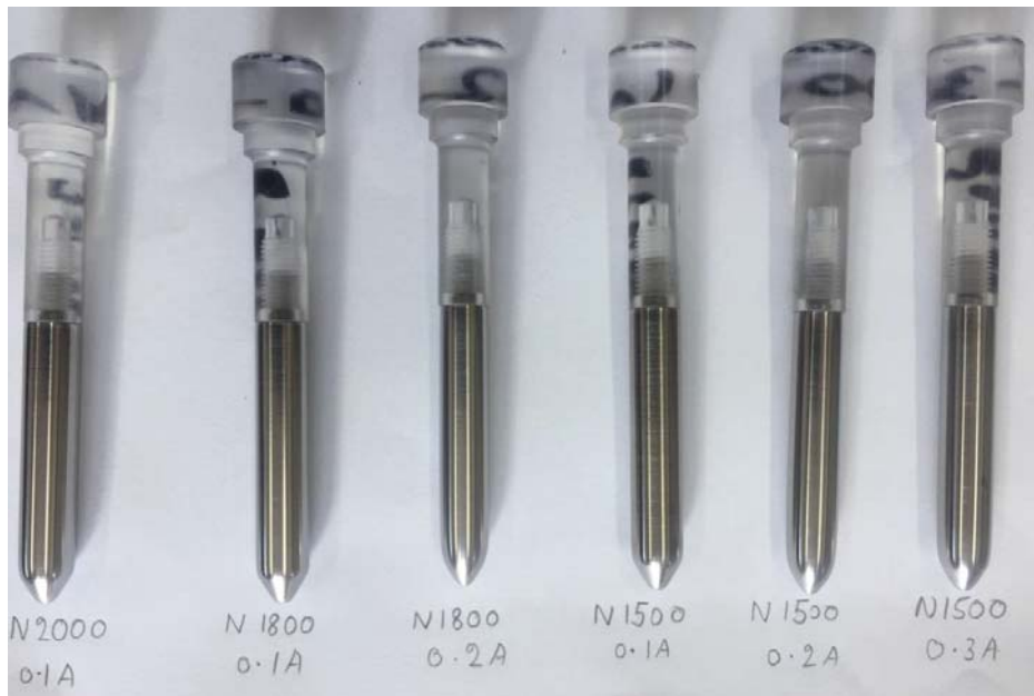
Figure 5.17: Performance rating of combination of Neem with Aminic antioxidants at different concentrations
