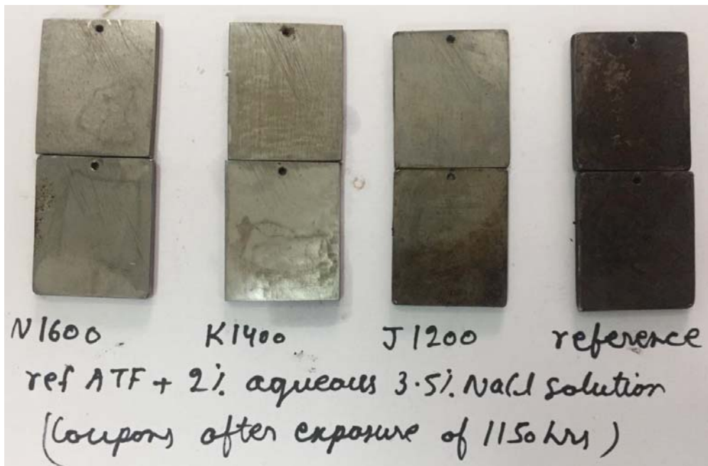
Figure 5.33: Coupons after testing with 2% volume of 3.5% NaCl after 1150hours
