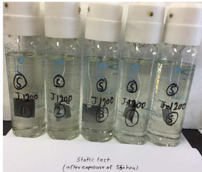
Figure 5.26: Test bottles containing coupons at the end of 550hours of static tests for 1200ppm of Jatropha
