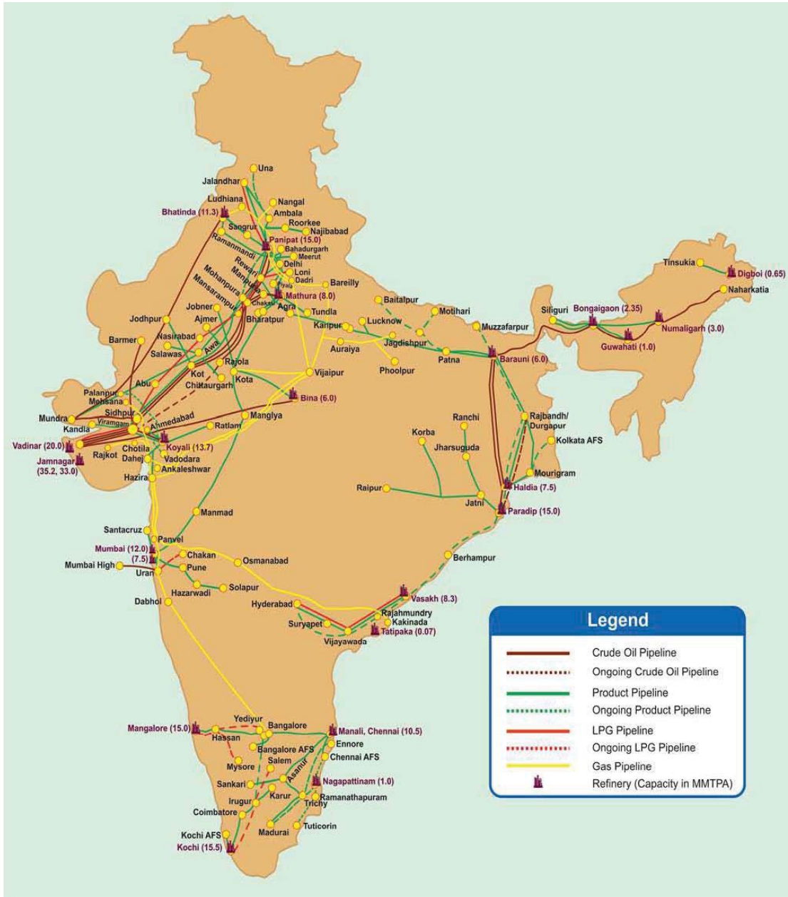
Figure 1.6: Petroleum pipeline network across the country (PPAC, 2018)
