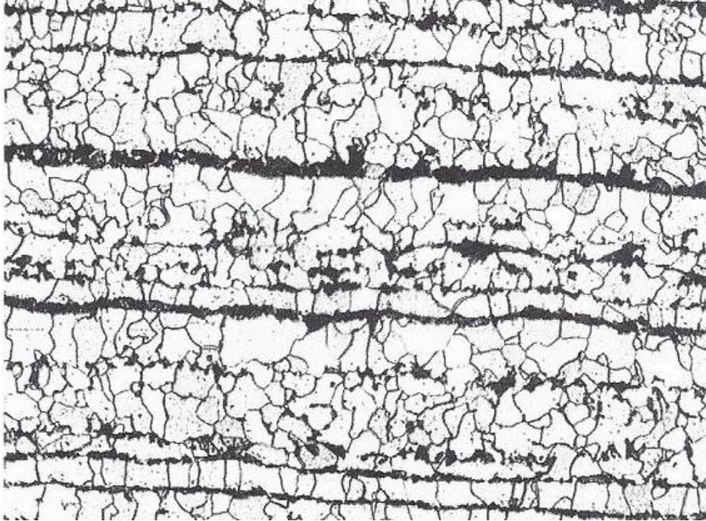
Figure 3.4: Sample D consists of ferrite-pearlite microstructure having large ferrite grains with different degree of carbide banding and grain growth.
