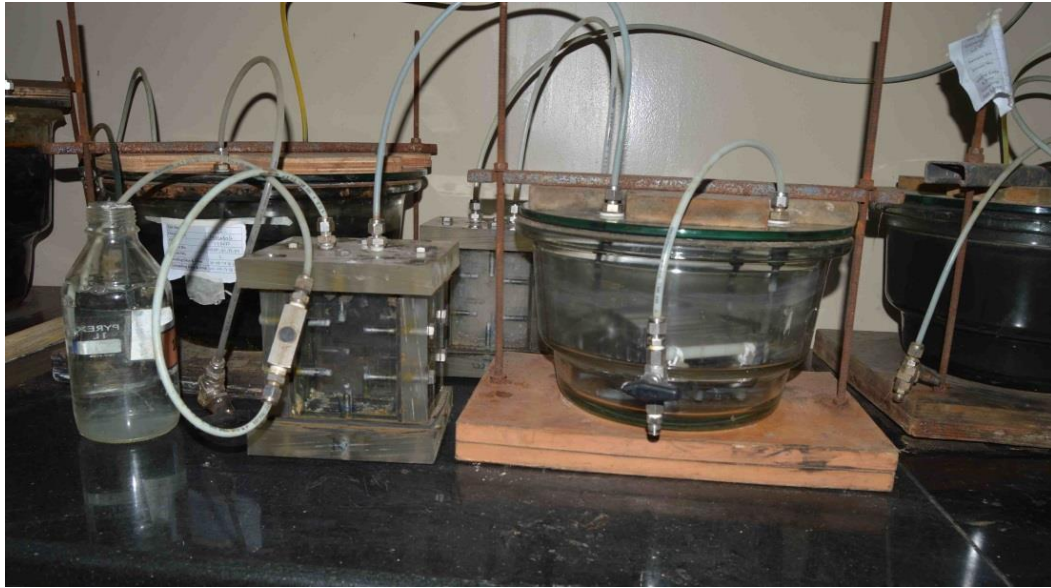
Figure 3.10: Photograph shows HIC test set-up in laboratory. Test specimens are placed in glass vessel immersed in test solution, H 2 S gas is continuously bubbled through the solution during testing.
