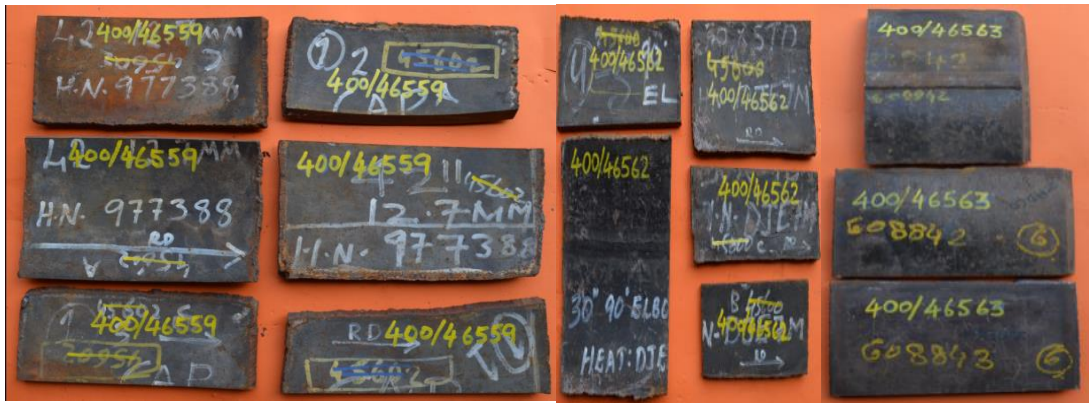
Figure 3.1: Sections cut from respective product as starting material for specimen preparation.
