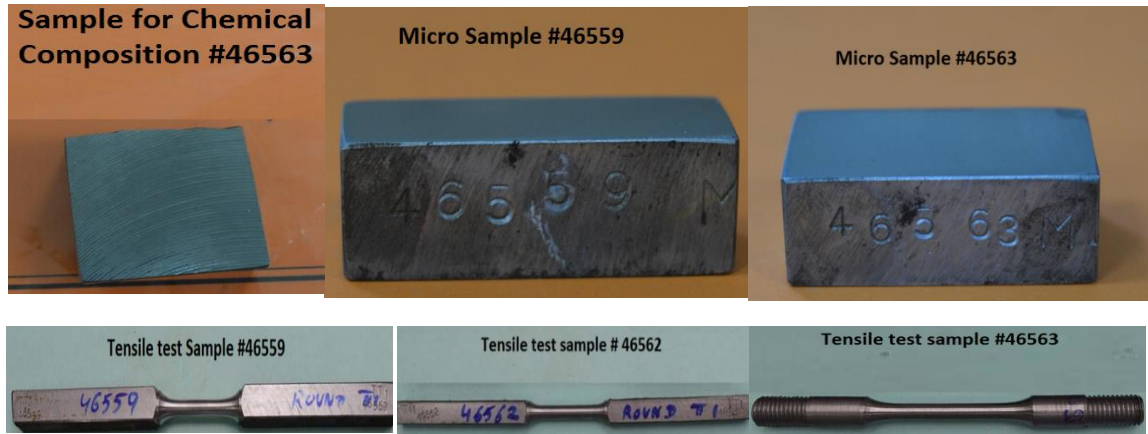
Figure 3.2: Photograph showing sample specimens prepared for testing.
