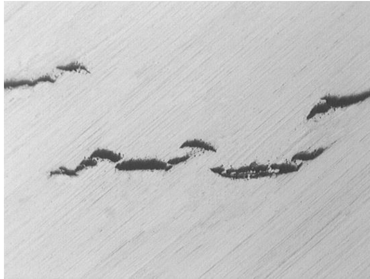
Figure 3.14: Metal sample-D, unetched surface showing HIC cracks (x100)
