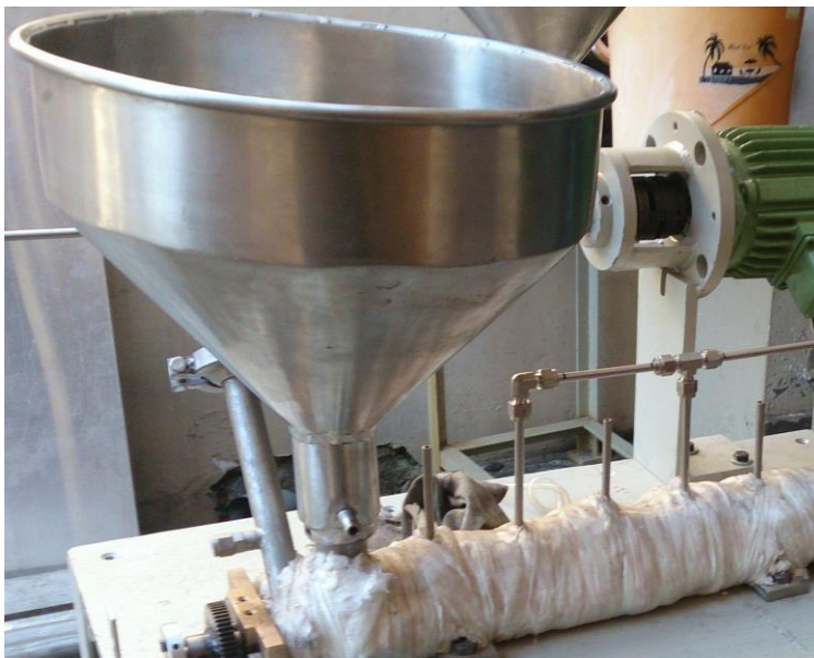
Fig 3.3. Biomass feeding hopper
