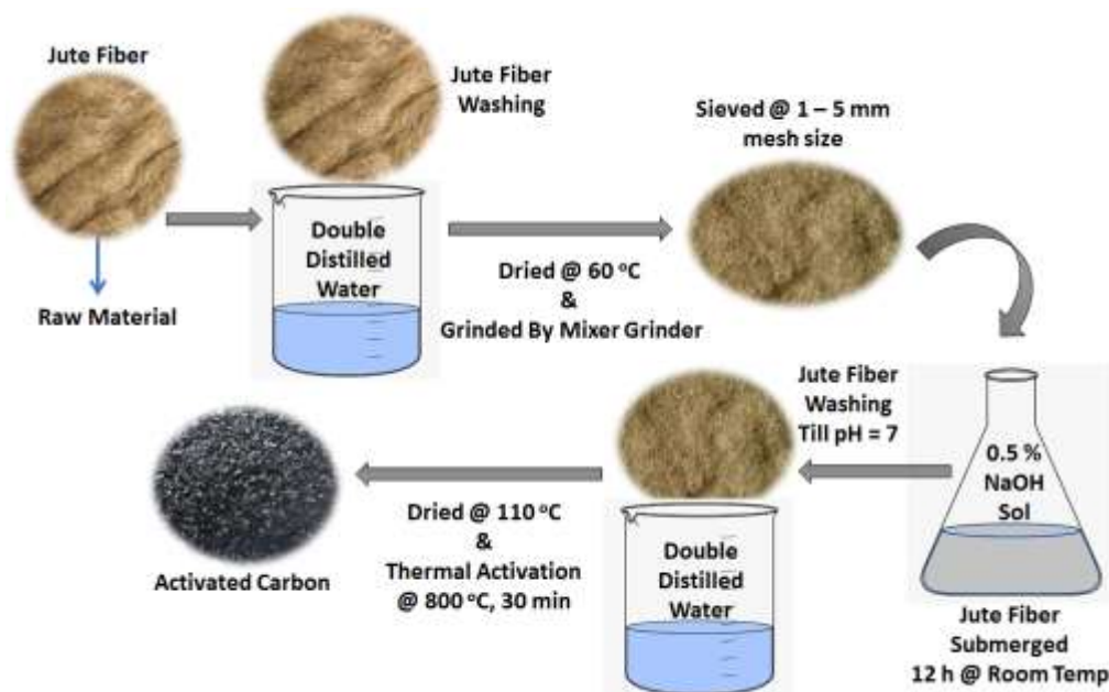
Fig 5.5 Activated carbon synthesis process using jute fiber
