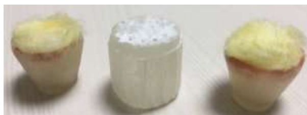
Fig 6.12 Titanium dioxide loaded parts of the model
