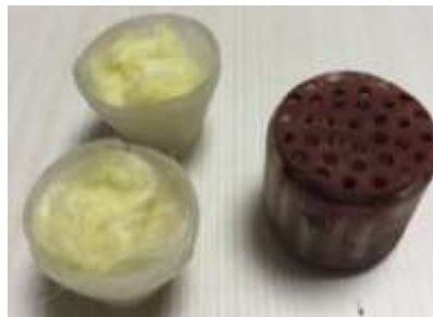
Fig 6.5 Hematite loaded parts of the model
