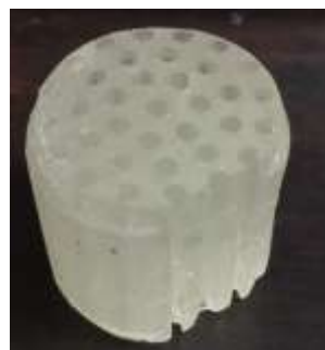
Fig 4.15 Cylindrical structure deformation
