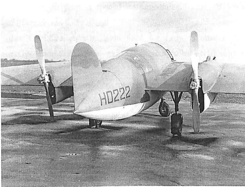
Figure 10.1: Push prop configuration [Source: Wikipedia]
