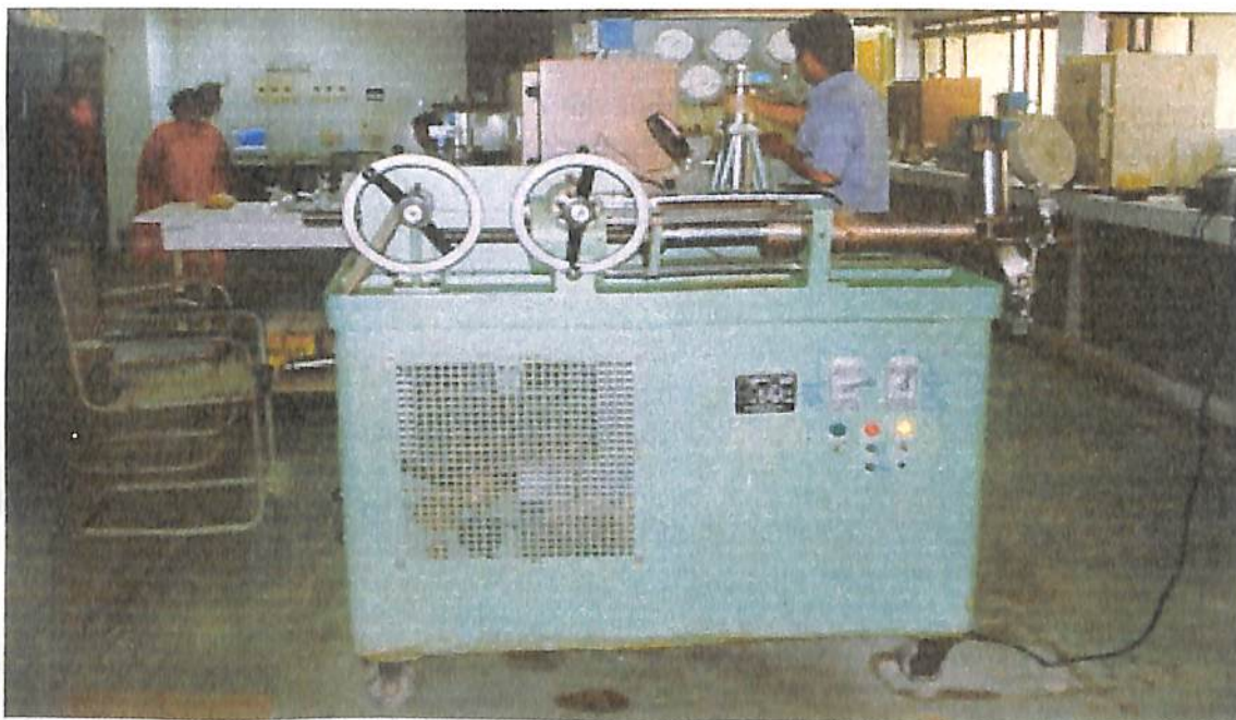
Coreflood Apparatus (RUSKA Proportionating Pump), Courtesy ONGC
