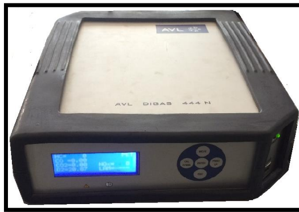
Figure 3.7: AVL DIGAS 444 gas analyzer
