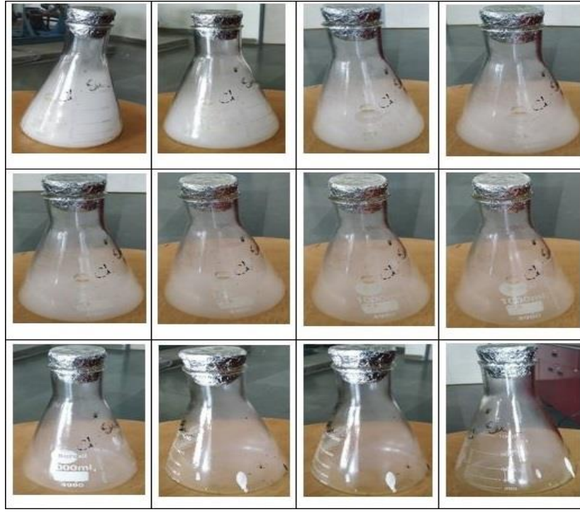
Figure 3.19: Diesel vapor at various time intervals of 10 seconds
