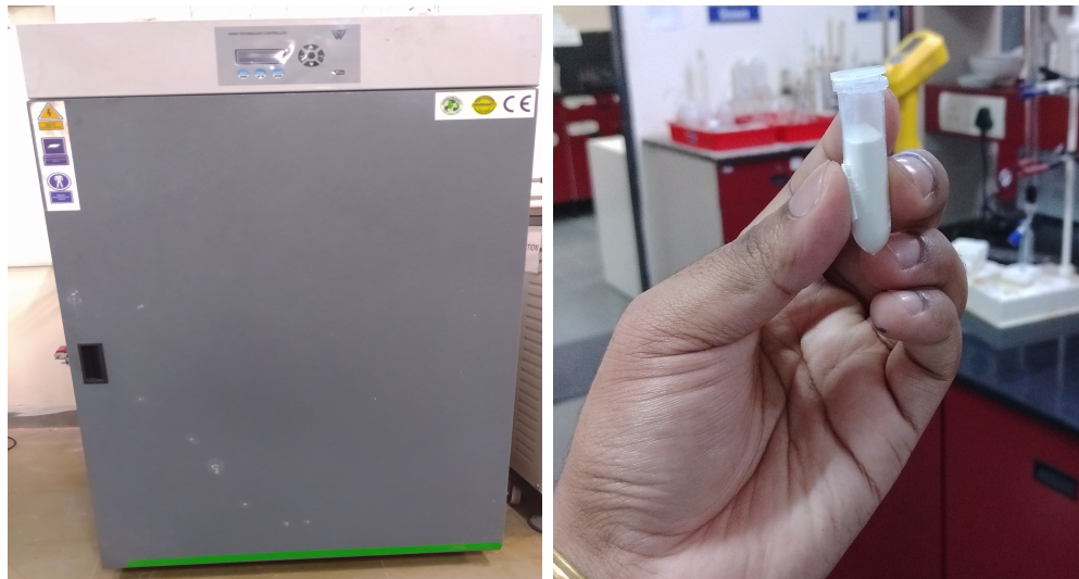
(c) The white precipitate is collected and heated overnight at 100 °C (d) Final TiO 2 powder is collected after manually grinding process.
