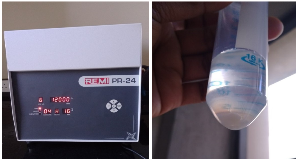
(a) The sample of white slurry solution is centrifuged for 20 min. at 12000 rpm (b) centrifugation separated the white precipitate collected at the bottom of the vessel
