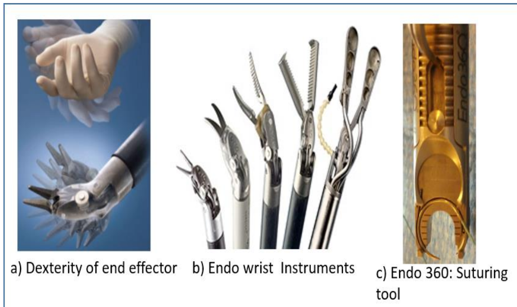
Figure 2.2: Different Types of End-Effector tools [36], [37]
