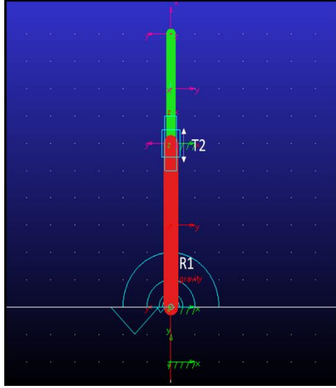
Figure 3.6: Structural Representation of a two-link RT configuration robot.
