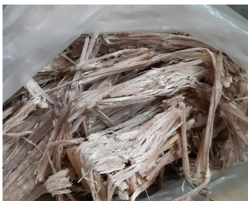
Figure 3.3. Clean and dry Sugarcane husk
