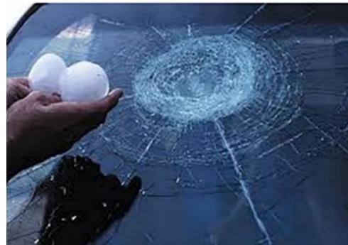
Fig2.30 Hailstorm affected PV module
