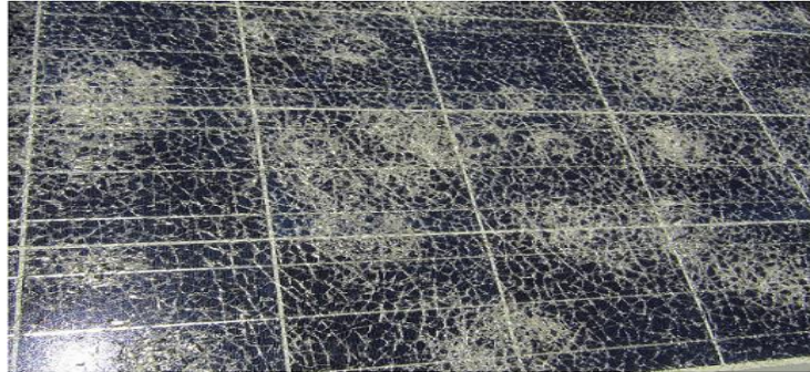
Fig.2.39 Module with broken glass after heavy hailstorm (plant 1) [164]
